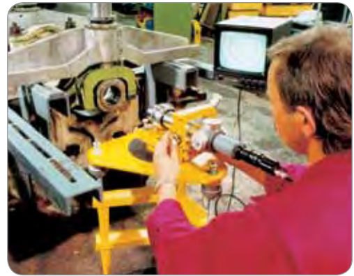
Diesel engine alignment (shown here using CCTV system 137-2161-01)
