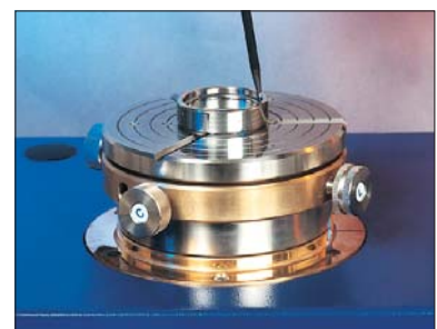
gauge arm in vertical attitude with orientation retracted to measure an inside diameter
