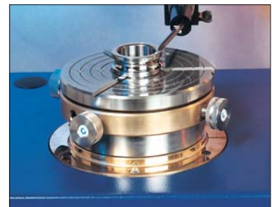
gauge arm in horizontal attitude with orientation downward to measure top face
